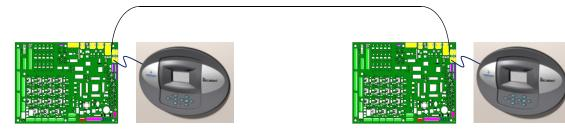
**Three or more units with small displays**: To network three or more cooling units, each equipped with a small display, connect a straight-through CAT5 Ethernet cable from the P64 connector on each cooling unit's Liebert iCOM input/output board to a common network switch (see **Figure 26**).
